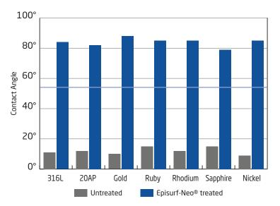
Oil contact angle on different materials before and after Episurf-Neo® treatment.
